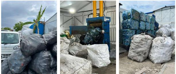
Figure 16: PET bottles bagged and baled for export at a recycler.
